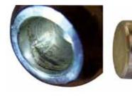
Fig. 4 Example of trunnionosis of a cobalt chromium femoral head and the tapered portion of the femoral prosthesis.
