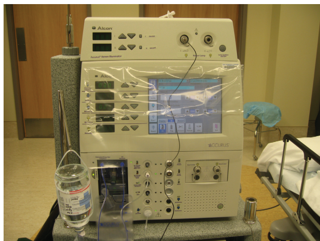
Figure 4. Photograph of the computerized vitrectomy console that contains the driver for the vitreous cutter, the fiber optic light source and the infusion pump.
